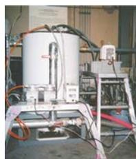
Reactor for aerobic denitrification
